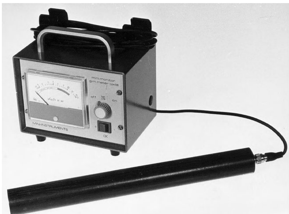
Figure 6.2. A Geiger–Mueller counter. The sensitive volume is a tube which is connected to a pulse counter. The counter yields information about the radiation intensity.
